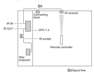
Connect the IR emitter to the DPC-7.4's IR OUT, and place the IR emitter in front of the other AV component's remote control sensor (usually located on its front panel), as shown below. See the instructions supplied with the IR emitter.
